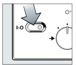
The rotary iron is turned on and off with the "I / 0" button.
